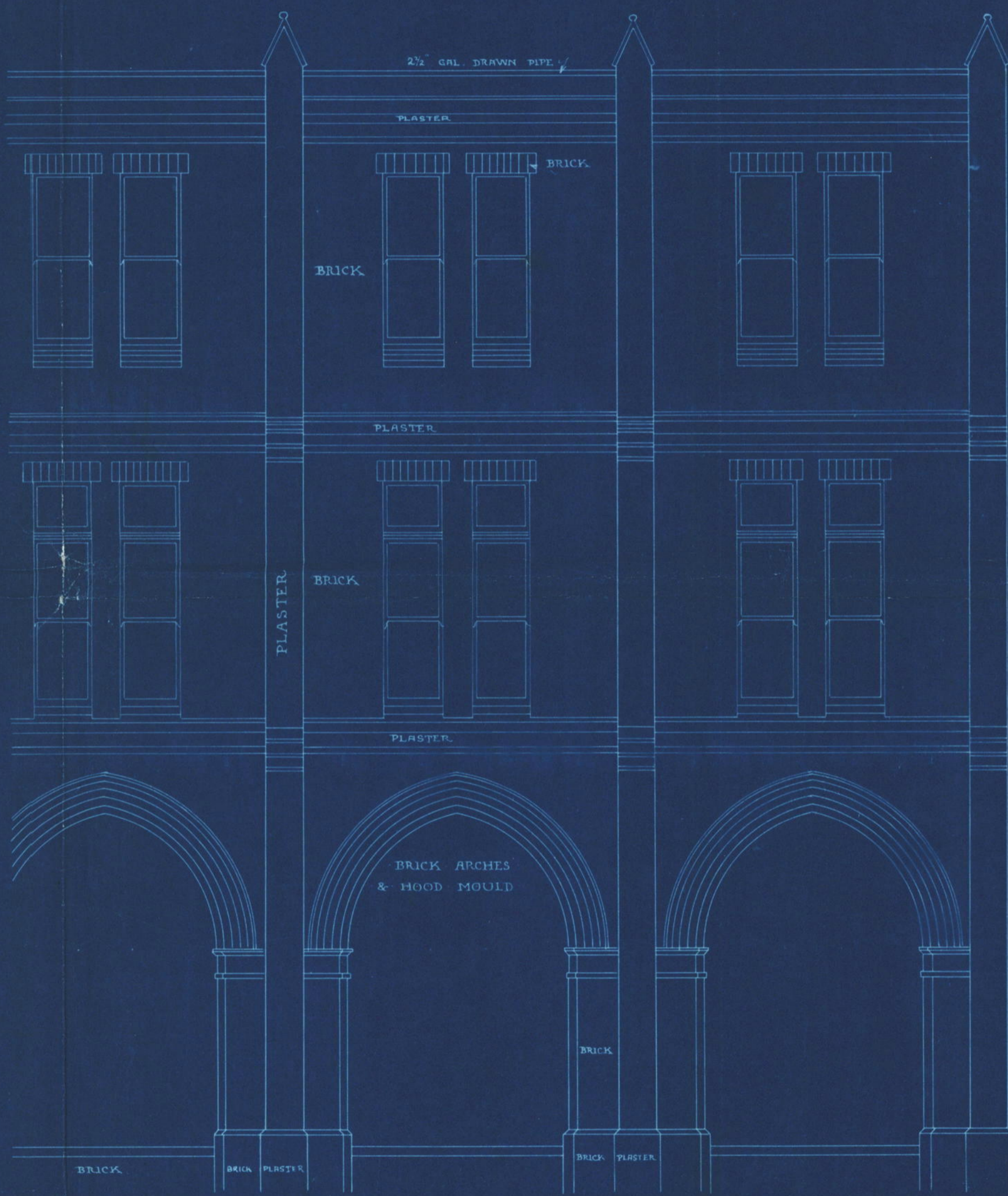
ELEVATION OF PART OF EAST ELEVATION SHOWING POSITIONS OF BANDS ETC. FOR FURTHER DETAILS SEE SHEET NO. 10
