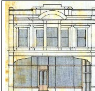
Detail from the original plans showing the Cuba Street elevation (WC Archives 00053:148:8200)
