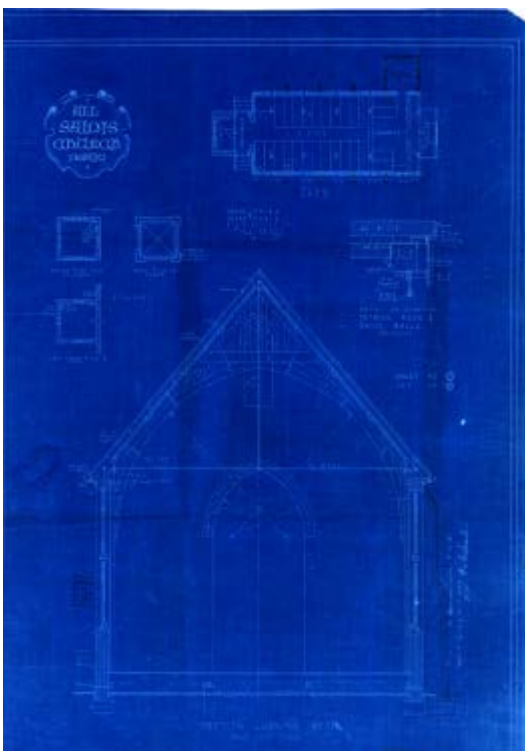
1928 Plan and section including first and second floor plans to the bell-tower and a detail of the connection between the brick nave walls and the timber cladding to the end sanctuary wall. All images: WCC archives
